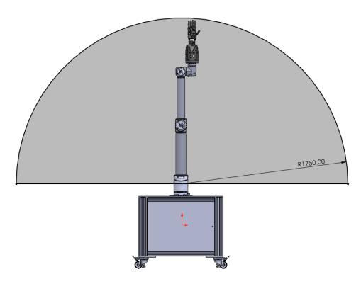
It should be noted that arm control is impaired at full extension, a universal problem in inverse kinematics, and the practical workspace of the arm is in fact slightly smaller than indicated.
